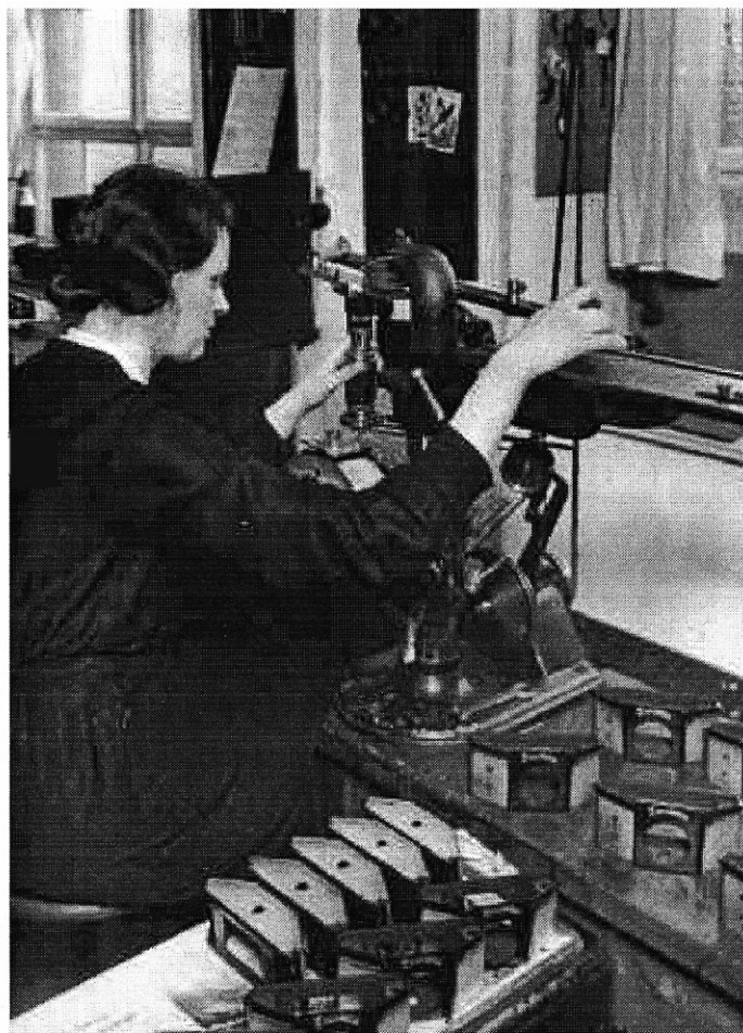
Engraving the name "Exakta" on VP Exaktas
