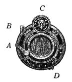
The **lbsor Shutter** shown here is also an automatic one which is always ready and requires no setting. Exposure is made by the depression of the finger release A or, if preferred, of the wire release which may be screwed into the small nut B.
