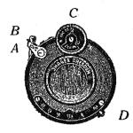
Shutter for time and instantaneous exposures  $^{1}/_{25}-^{1}/_{100}$  sec. The **Zenith Shutter** shown is of the automatic type, i. e.: it is always ready and need not be set. Exposure is made by depressing the finger release A or, if preferred, the wire release which can be screwed into the small put B.
