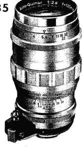
The f/2.8, 135 mm Auto-Quinar Telephoto lens with instant-reopen automatic diaphragm is a fast telephoto lens of superior design. Comprised of a 5-element lens system, this lens meets the highest standards for color, sharpness and performance. There are 8 diaphragm stops from f/2.8 to f/32. Angle of view is 18°. Lens focuses from infinity down to 5 feet, and can be operated both automatically and manually. Leather case and sunshade furnished with lens at no additional charge.
