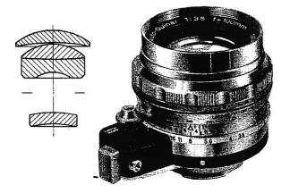
The fascinating f/3.5, 100 mm Auto-Quinar with instant-reopen automatic diaphragm is a true telephoto objective. It assures exceptional light intensity, unique brilliance, and needle-sharp critical definition. This lens combines the features of a normal and a telephoto lens, making it most desirable where natural proportions and perspective are essential. The angle of view is 27°. The diaphragm stops down to f/32; focuses from infinity to 3.8 feet. Lens operates both automatically and manually.
