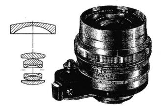
The renowned 7-element f/2.8 Auto-Quinaron 35 mm Wide Angle lens has an instant-reopen automatic diaphragm. It focuses from infinity down to  $4^{1/2}$  inches from the front element of the lens to the subject. Does not require bellows extensions or extension tubes for closeups. The angle of view is  $62^{0}$ , smallest of 7 diaphragm stops is f/22. Lens can also be operated manually if desired.
