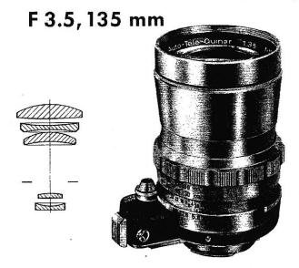
The f/3.5, 135 mm Auto-Tele-Quinar Telephoto lens with instant-reopen automatic diaphragm is a new 5-element objective in a light-weight chrome mount. The lens will give high performance to meet the demanding requirements of the 'perfectionist'. There are 8 diaphragm stops from f/3.5 to f/32. Angle of view is 18°. Lens focuses from infinity to 6¹/2 feet, and has dual control for both automatic and manual operation. Leather case and sunshade furnished at no additional charge.
