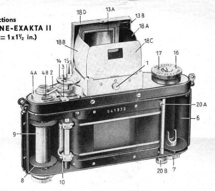
Changing lenses: After pressing the lens catch (19) lightly towards the lens and simultaneously turning the lens to the left as far as it will go, the lens can be lifted from the camera-body. The new lens is held into the lens mount so that red mark on the lens comes to lie against the red dot on the camera body. Now the lens is turned firmly to the right until the lens catch (19) is heard to slip into the catch on the lens mount.
