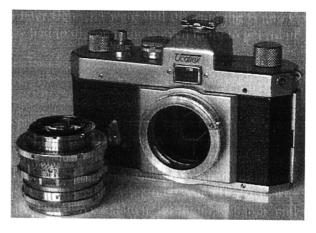
The lens mount is threaded M40. For Exakta lenses there was a special connector. Usually it is impossible to have a ring to connect M40 to Exakta properly, but because the camera is so thin, there is space available between the body and the Exakta mount lens, allowing focusing
