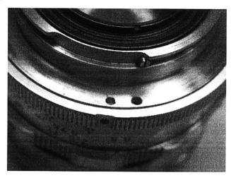
Exakta mount lenses can be used on this camera, but the little locking screw at the rear of the lens has to be removed first. The Ucaflex has its own lens locking mechanism.
