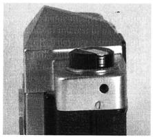
However, the shutter is as simple as in an old roll film box: 1/125sec (on the Plusflex an extra 1/60) and B. Its construction is in principle the same as the shutter of the Exa, with mirror and metal sector working together. The manual calls this a focal plane shutter. It is the secret to the low cost, the lack of mirror shock or vibration, and the lowest noise level of any single lens reflex camera.
