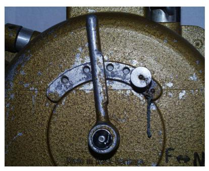
from the outside. Nevertheless, the housing does offer a pre-set function. The long aperture lever can be turned along a quarter-circle metal rim with six holes. A pin, connected to the housing by a little safety chain, can be put in the appropriate hole (2.9 - 4 - 5.6)– 8 – 11 – 16). Without looking, one can turn the diaphragm open or shut. Left is open, right to stop against the pin is closed. The maximum aperture of 2.9 already suggests the use of a Meritar, even
