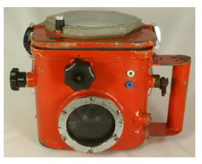
The interior is rusty and stinks, so the seals are clearly not what they ought to be. The focussing mechanism is quite complicated, with five cogwheels and a corrugated iron band around the lens. The first two cogwheels were connected by a chain, but unfortunately that is rusted and broken.
