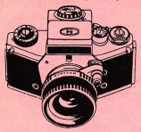
Suitable for all models of Exakta, this through the lens metering system is built into a pentaprism which is interchangeable with any of the existing viewing systems. C.D.S. meter mounted above the viewfinder correctly reads irrespective of lens focal length, mechanical extensions (bellows, tubes etc.) or filters, and translates visually in the viewfinder by a simple needle/zero line up.
