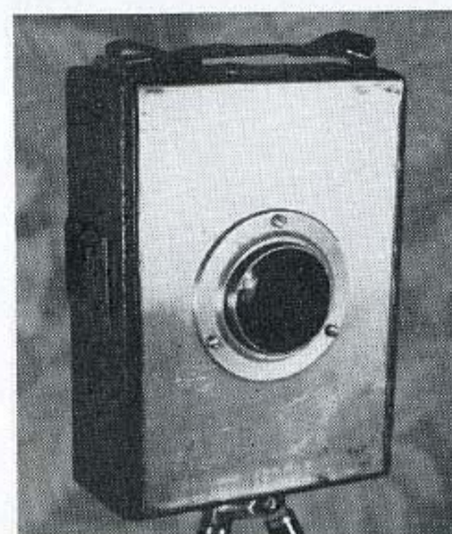
Paul Wolf's "dream camera", shown at the left, is a combination of an Exakta and a 9x12 camera with a bellows. The back of the 9x12 camera is adapted as shown below to take the Exakta. Wolf prefers this combination for taking close-up photos in color so he can use the bellows.
