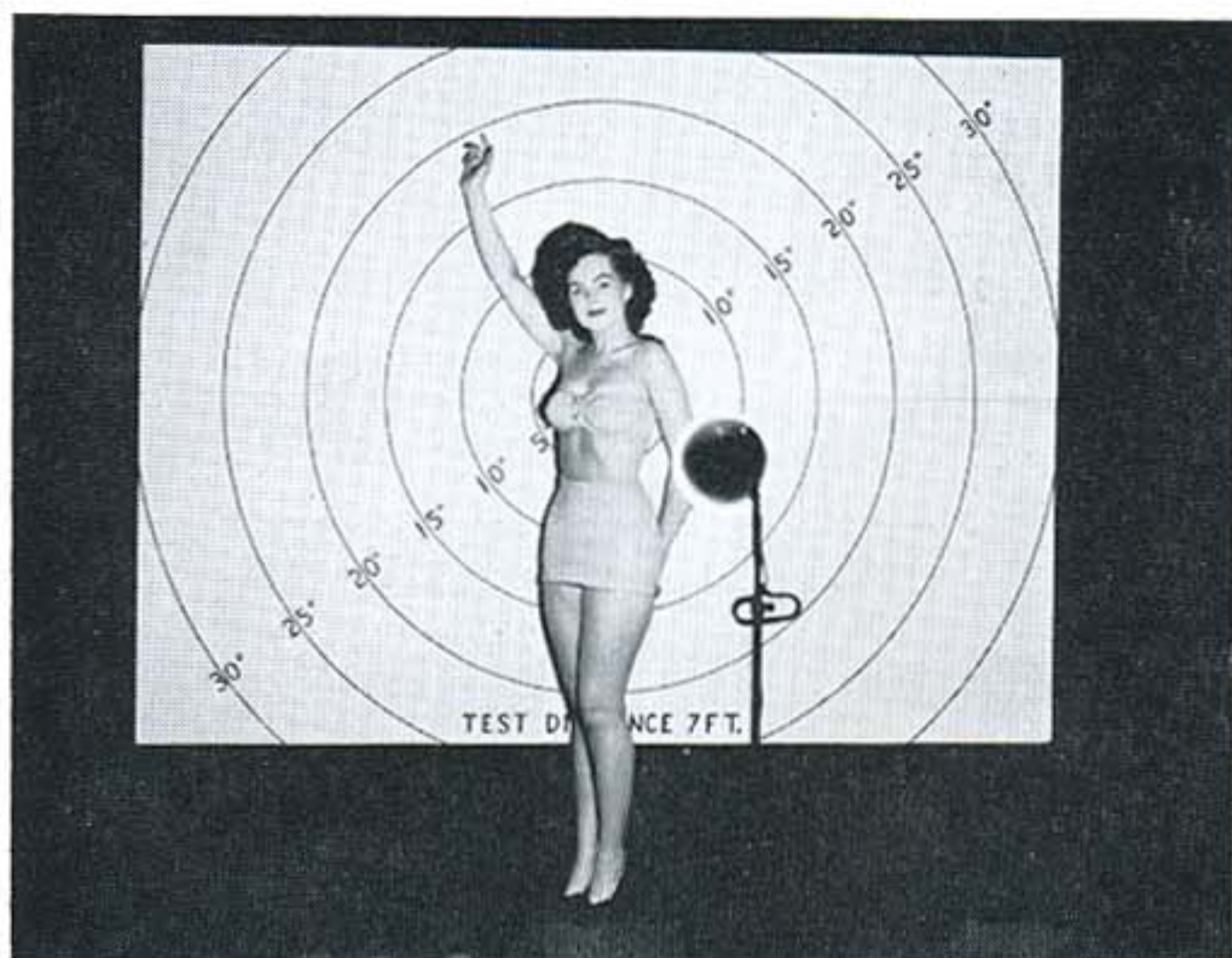
Relative angle of coverage of G.E.'s RFL2 is shown above. Note wide, smooth spread of light. Reflector flood's beam is about 90°.
