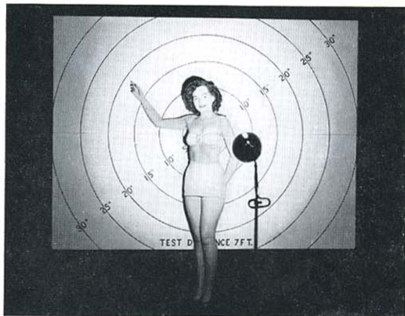
G.E. claims only 40° coverage for the 375-watt medium beam reflector floodlamp but target shows about 50° is well-lighted.
