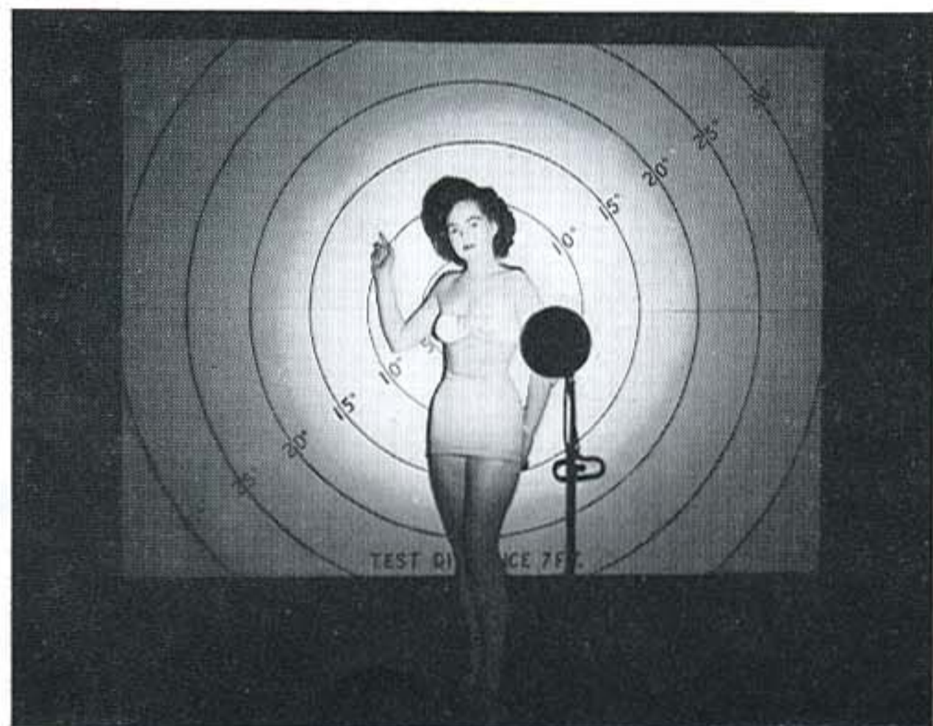
Intense concentrated beam of RSP2 is shown here. Coverage is only 20° but light intensity is nearly eight times that of RFL2.
