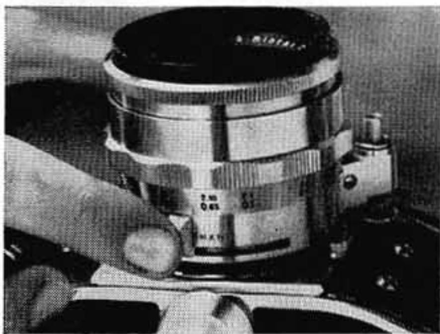
Sweep lever underneath Zeiss Biotar barrel opens diaphragm to f/2 for focusing after each shot. Lens can be used manually by ignoring this lever.
