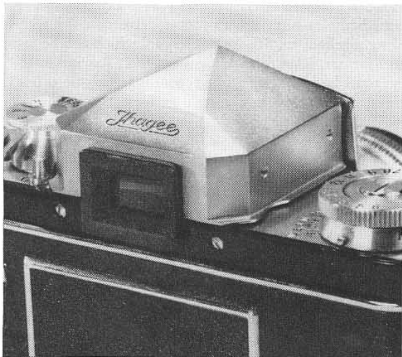
The Exakta Penta Prism eye-level prismatic viewfinder, above , is instantly interchangeable with the waist-level finder which comes with the camera. After light enters the camera lens, below , it hits a mirror placed at a 45 degree angle to the film plane. The light image is then reflected to the Penta Prism. As the image bounces and is reflected off the top and front of the prism, it is enlarged, corrected right to left, and reflected to the eye for focusing and for viewing.
