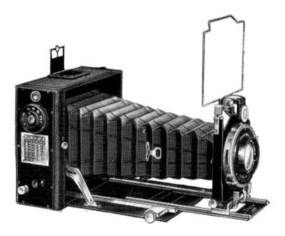
The Focal Plane Duplex is a horizontal model fitted with the IHAGEE patented Self-Capping Focal Plane Shutter, giving a range of speeds from 1/15th to 1/1000th of a second and working entirely without vibration. It is also fitted with a Compur Shutter with delayed action, giving speeds from 1 second to 1/250th second. The Focal Plane Duplex is, therefore, a truly universal instrument, capable of every class of photographic work.
