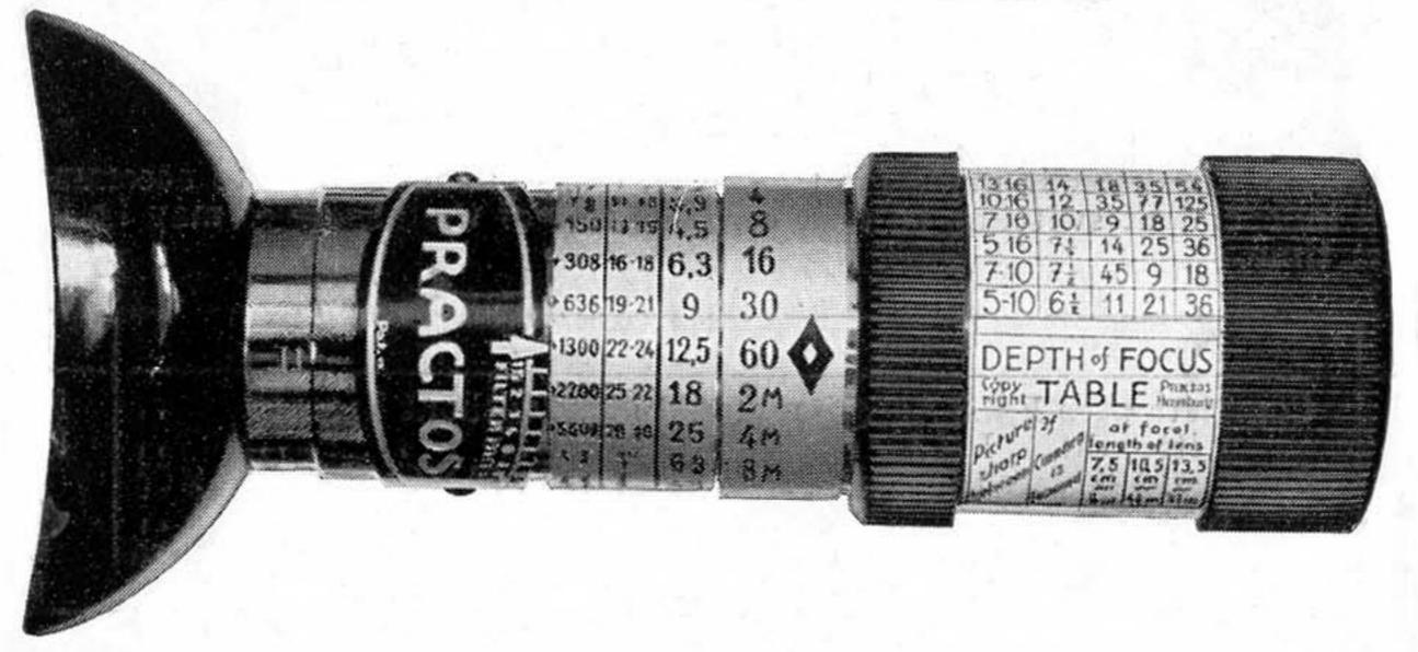
The Practos is the latest, most interesting and most efficient of this type of Exposure Meter. It is so simplified that after adjusting the Eyepiece to suit one's vision, it is only necessary to look through it and turn the rotating ring until the figure on the left is obliterated, when the actual exposure desirable will appear on the right hand side.
